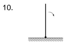
A thin uniform rod of mass *M* and length *L* is positioned vertically above an anchored frictionless pivot point, as shown above, and then allowed to fall to the ground. With what speed does the free end of the rod strike the ground?
